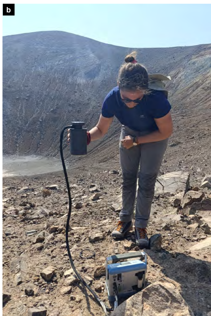
(a) Cinzia Federico (INGV-Palermo) explaining how to collect fumarolic gas samples at Baia di Levante, Vulcano; (b) A participant measuring CO 2 degassing of La Fossa Crater (Vulcano) using an accumulation chamber
