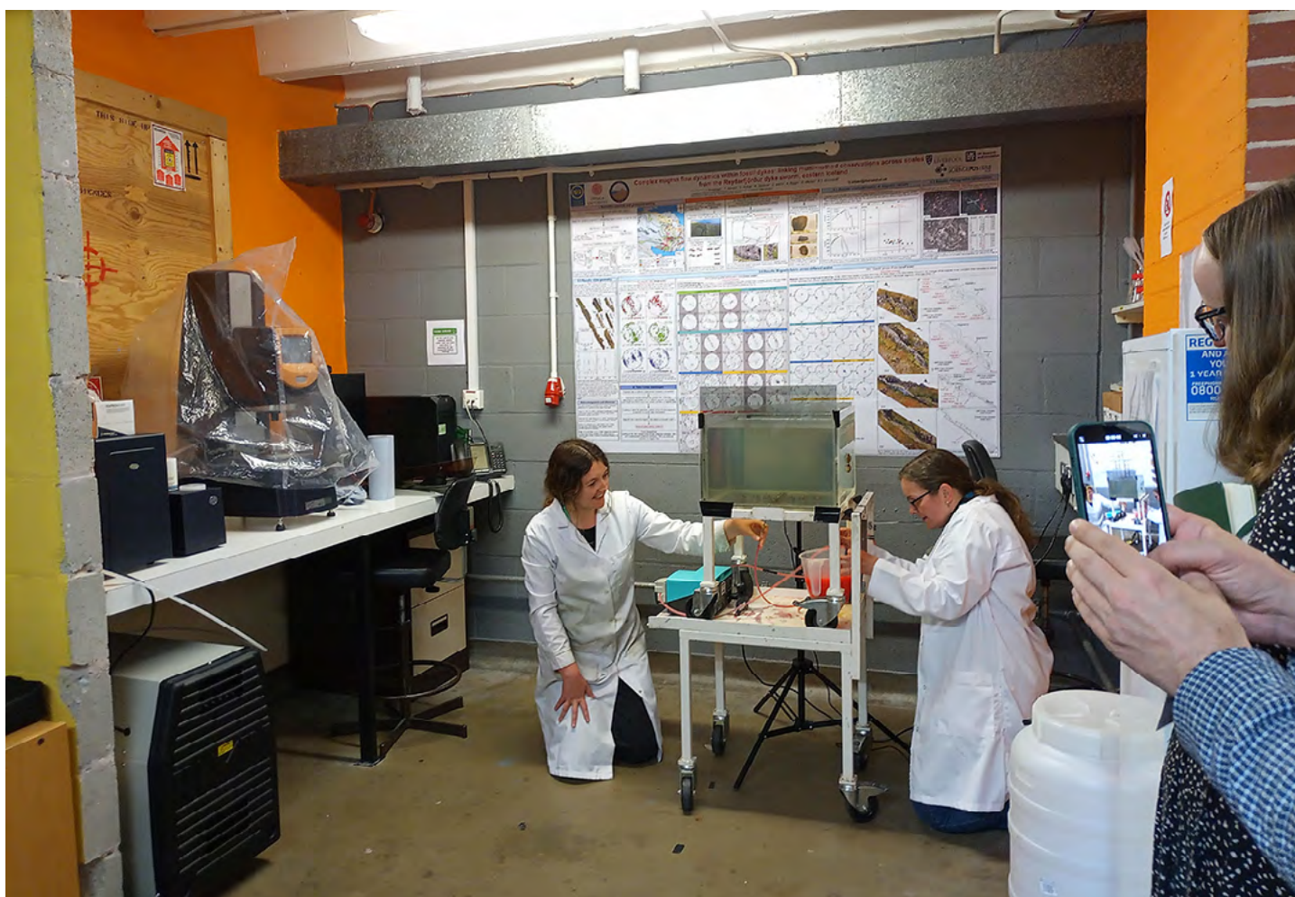
Demonstrations in the Magma Lab. Based in the University of Liverpool's Jane Herdman Building, the facility is designed for analogue modelling experiments, namely particle image velocimetry and digital image correlation relating to fluid dynamics, magma flow, and volcanic plumbing systems ( https://www.liverpoolmagmalab.org/facilities )
