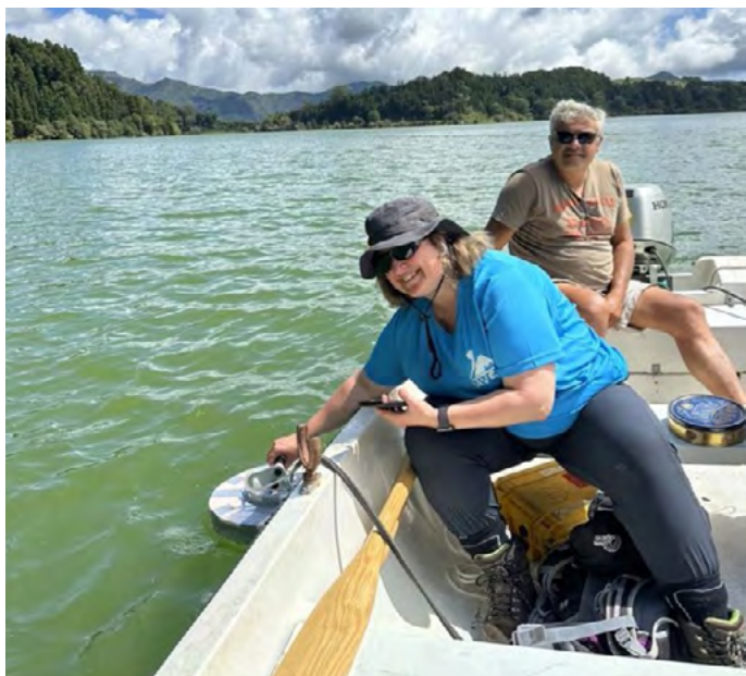
Furnas Lake fieldwork: CO 2 flux measurements with Agnes Mazot
