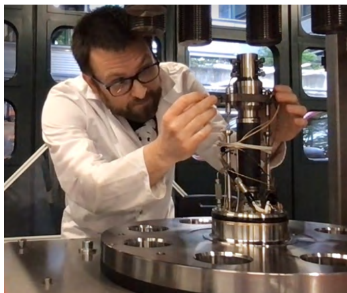
Mike setting up a triaxial deformation experiment in the laboratory
